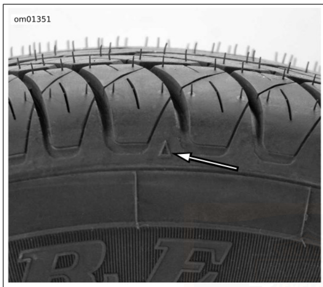
Figure 59. Rear Tire Tread Wear Bar Indicator VEHICLE ALIGNMENT
