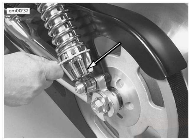
Figure 11. Adjusting Rear Shock: VRSC Models
