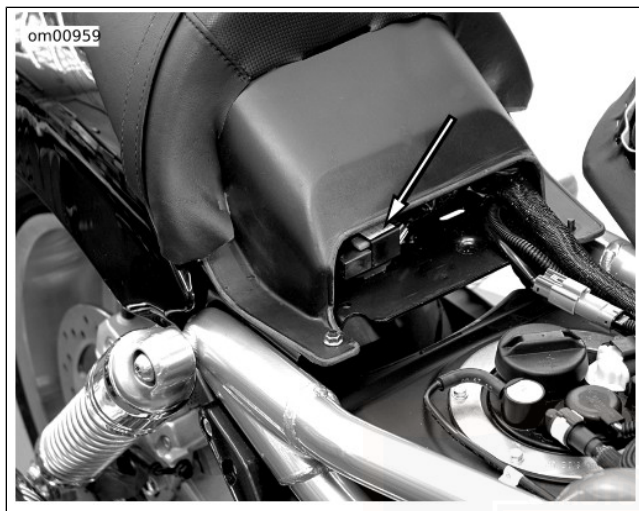
Figure 62. Rear Fuse Block Location: VRSC Models Except VRSCR
