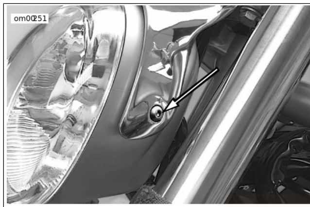
Figure 46. Headlamp Alignment Fastener: VRSC Models
