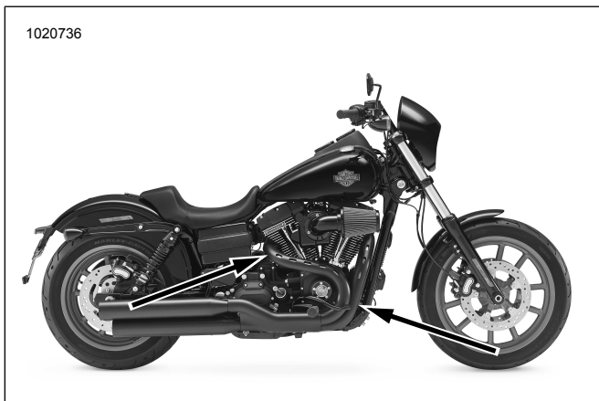
Figure 40. Oxygen Sensor Locations (Inboard Side of Exhaust Pipes)
