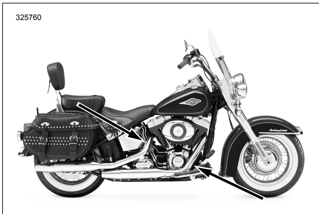
Figure 33. Oxygen Sensor Locations (Inboard Side of Exhaust Pipes)
