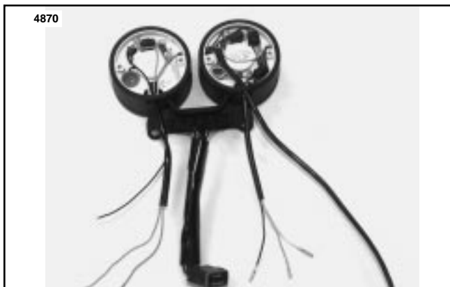
Figure 7. Speedometer (r) and Tachometer (l) Installed in Double Bracket (Rear Covers Removed for Illustration Purposes)
