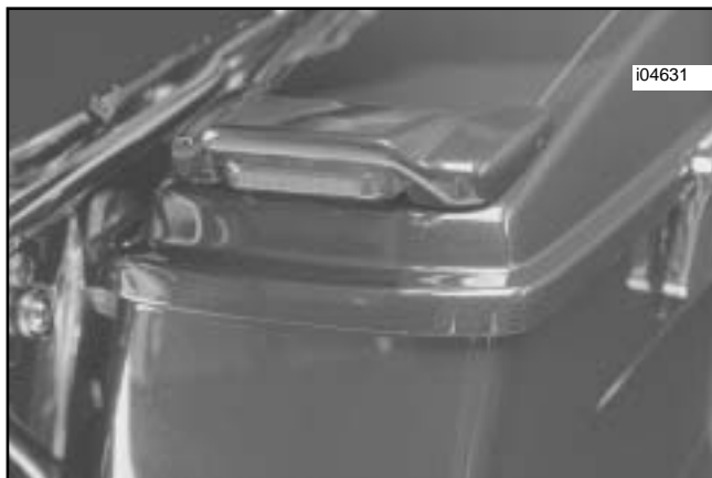
Figure 1. Installed Saddlebag lid spoiler
