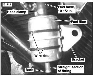
Figure 3. Filter Mounted to Bracket
