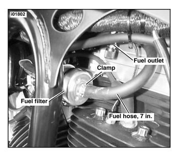
Figure 5. Fuel Tank to Filter
