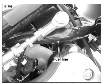
Figure 2. Fuel Line Routing
