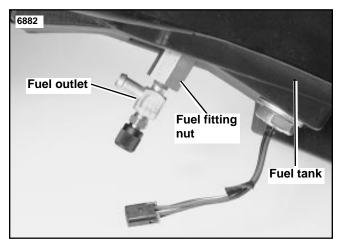
Figure 1. Fuel Outlet Fitting, Original Setup
