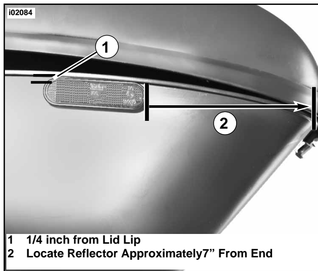
Figure 18. Install Reflectors to Saddlebags
