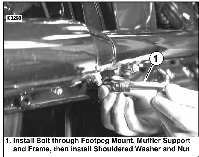
Figure 13. Saddlebag Support Bracket and Frame (2000 and Later Models)
