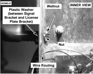
Figure 11. Turn Signal Installation (Left Side Shown)
