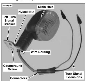
Figure 10. Pre-assemble Turn Signals (Left Turn Signal Shown)
