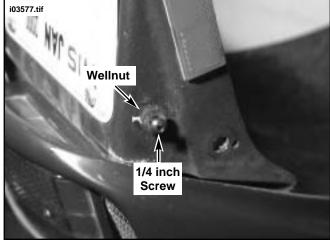
Figure 9. Install Rubber Wellnuts
