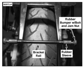
Figure 5. Install Rubber Sleeves and Bumpers
