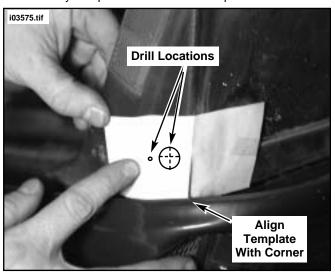
Figure 7. Proper Drill Template Orientation
