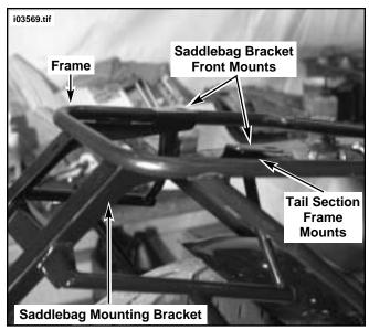
Figure 1. Position Front Upper Portion of Saddlebag
