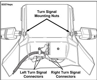
Figure 6. Remove Existing Turn Signal Assemblies
