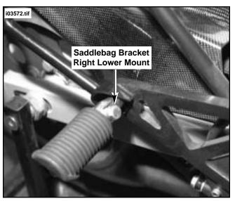
Figure 4. Re-install Passenger Footpegs (Right Shown)
