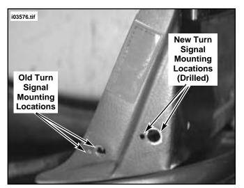
Figure 8. New Turn Signal Mounting Locations
