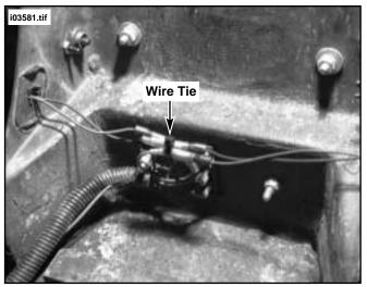
Figure 12. Connect Turn Signal Wiring
