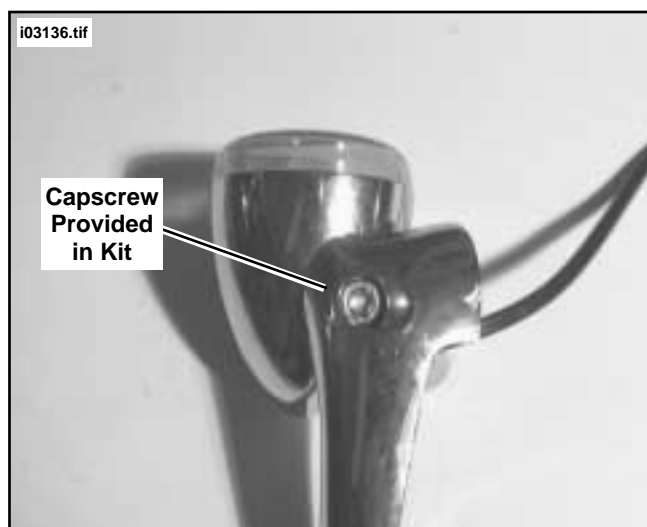
Figure 9. Install Turn Signal to Relocation Mount
