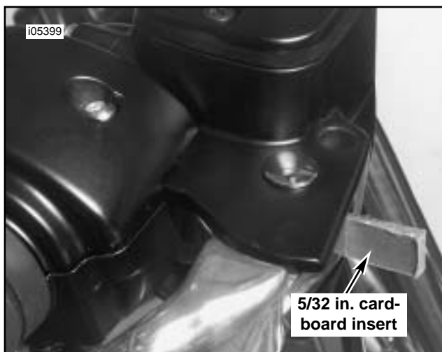
Figure 2. Install Insert Before Removing Master Cylinder
