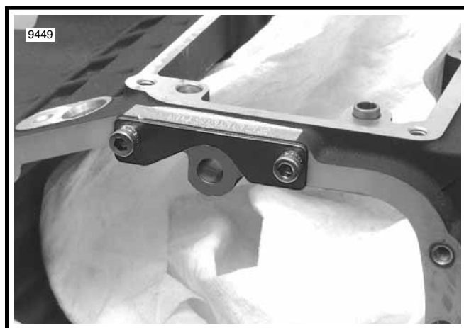
Figure 1. Install Drill Plate to Transmission Case
