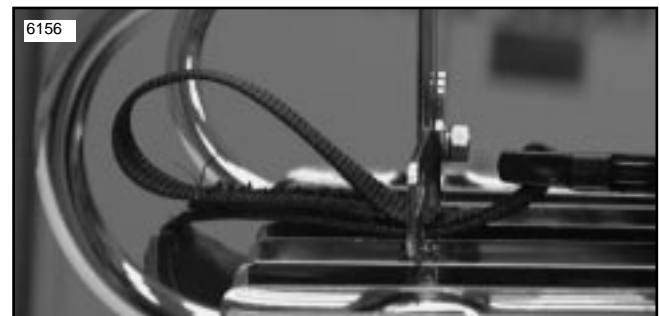
Figure 7. Fold excess strap length back onto velcro (shown on rack 53391-94)
