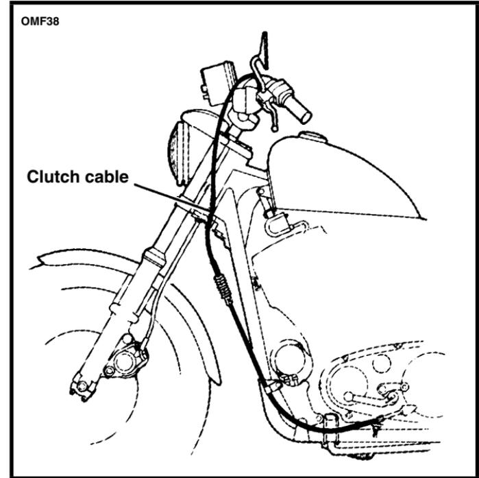
Figure 39. Clutch Control Cable (Typical)
