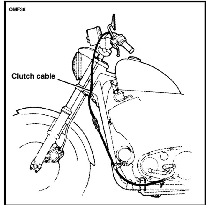
Figure 39. Clutch Control Cable (Typical)
