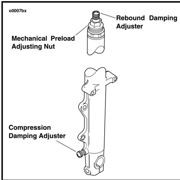
**Figure 21. Front Suspension Adjustments**
