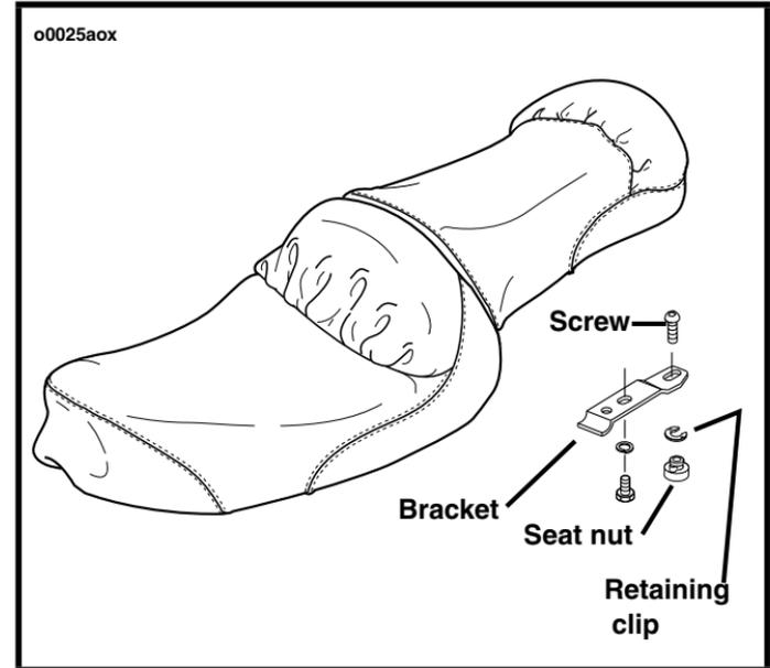
**Figure 47. Seat and Mounting Hardware (Typical)**
