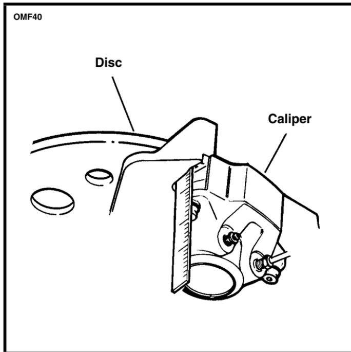
**Figure 41. Measuring Rear Brake Outer Pad - 1340cc Models**
