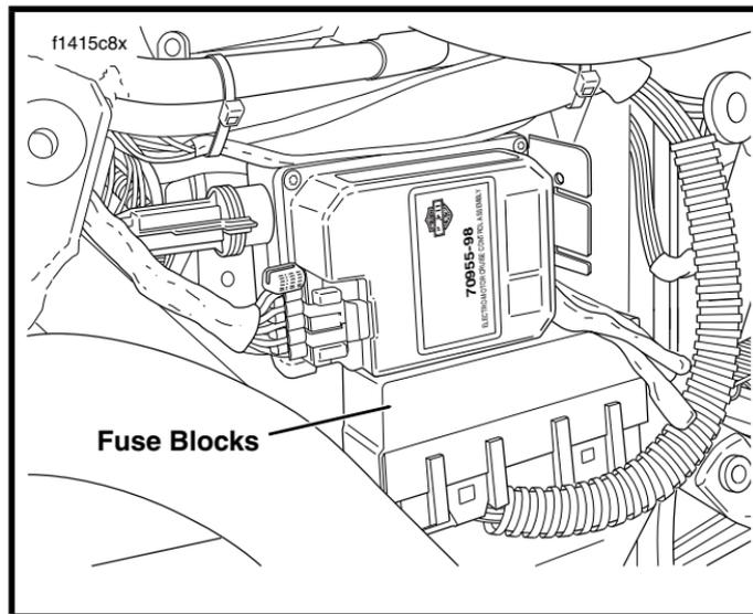
**Figure 49. Left Side Cover Removed - FLHTCU**
