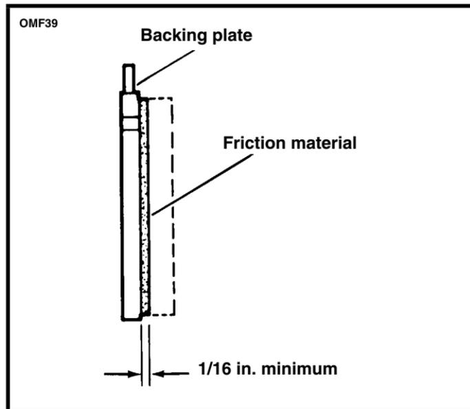
**Figure 40. Brake Pad - Side View**
