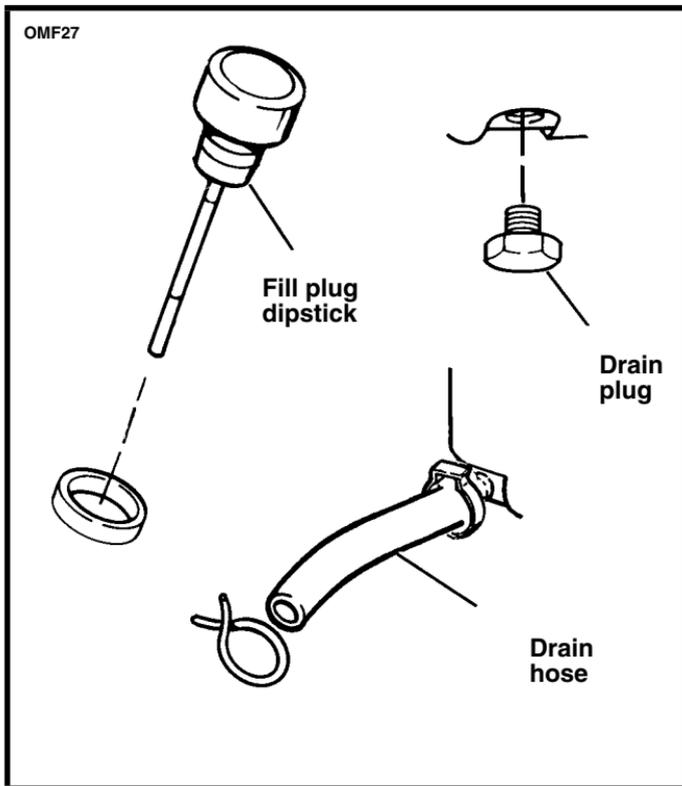
Figure 31. Fill Plug Dipstick & Oil Tank Drains
