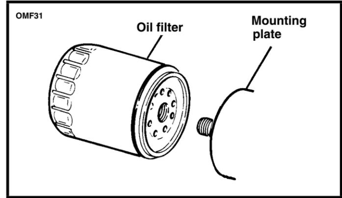
Figure 33. Engine Oil Filter
