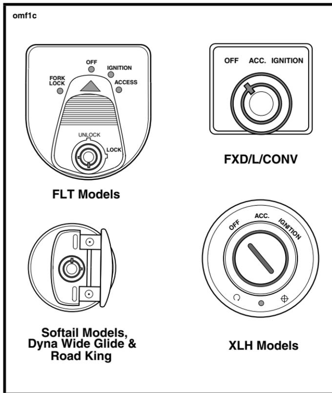
Figure 1. Ignition/Light Key Switch
