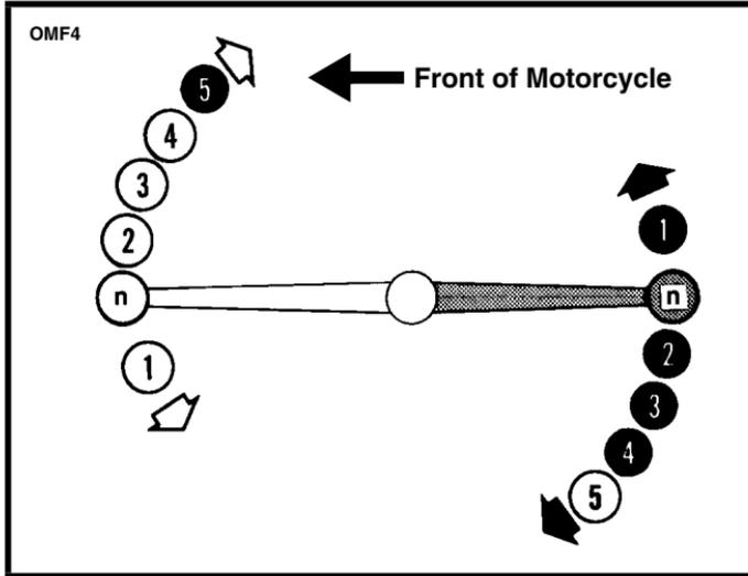
Figure 4. Gear Shifter
