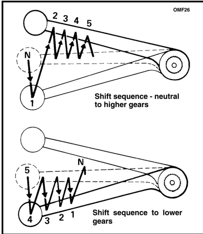
**Figure 30. 5 - Speed Shifting Sequence**
