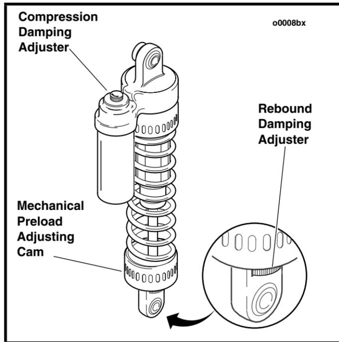
Figure 22. Rear Suspension Adjustments
