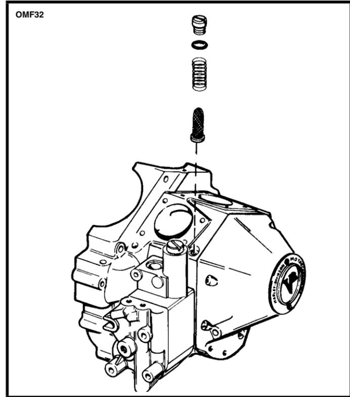
**Figure 34. Hydraulic Lifter Oil Filter Screen**
