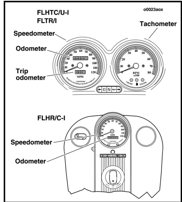
Figure 9. Speedometer, Odometer, Trip-odometer, Tachometer
