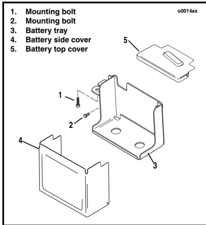
**Figure 48. Dyna Glide Battery Tray and Mounting Hardware**
