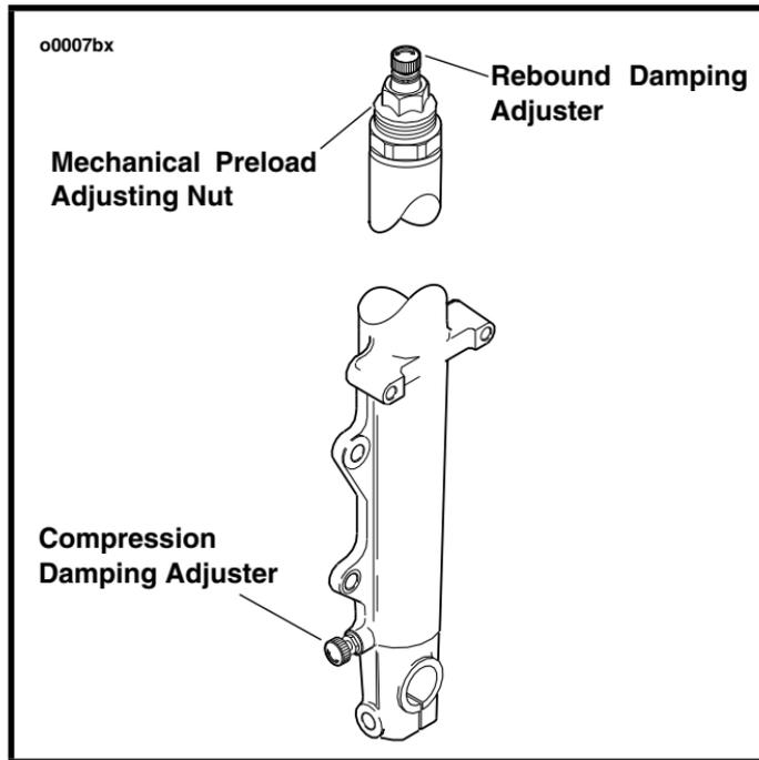
**Figure 21. Front Suspension Adjustments**
