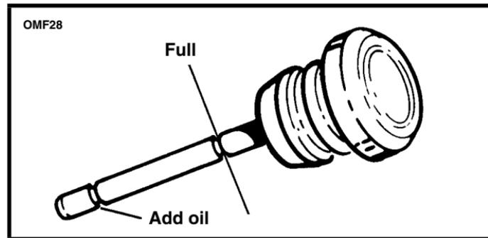
Figure 32. Engine Oil Level - XLH and Softail Models
