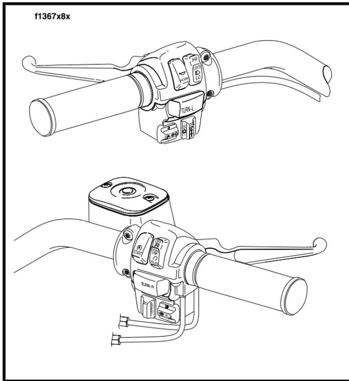
**Figure 6. Sound System/Cruise Control Handlebar Controls**
