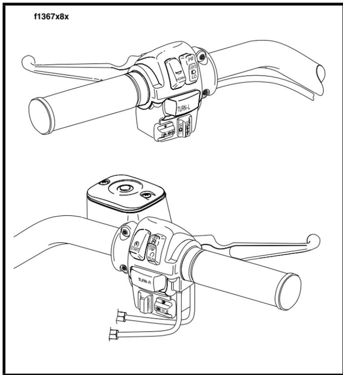
**Figure 6. Sound System/Cruise Control Handlebar Controls**
