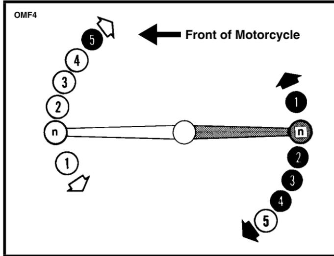
Figure 4. Gear Shifter
