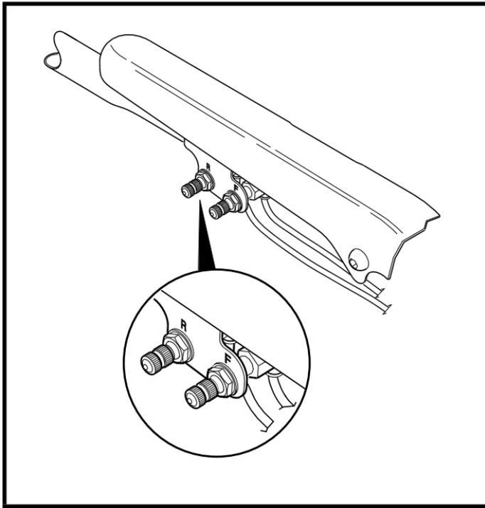
Figure 17. Air Suspension Adjustment Valves - FLT Models
