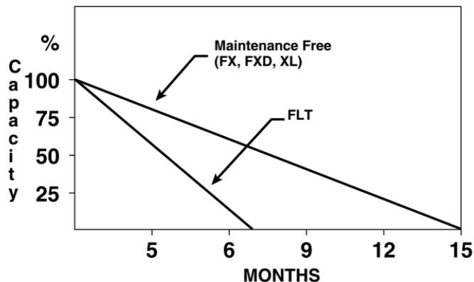
To reduce battery self discharge, remove and store the battery in a cool, (not freezing) dry place when the motorcycle is being stored.
