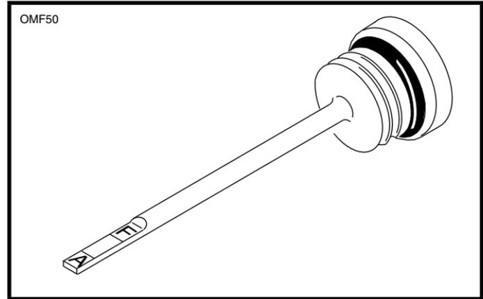
**Figure 35. Transmission Lubricant Dipstick - 1340cc**
