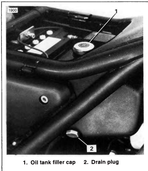
Figure 19. Oil Tank -- FXR
