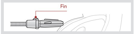
3. Attach the headset main unit to the clamp unit. Slide the main unit down onto the clamp unit until it clicks firmly into the bottom portion of the clamp unit.
