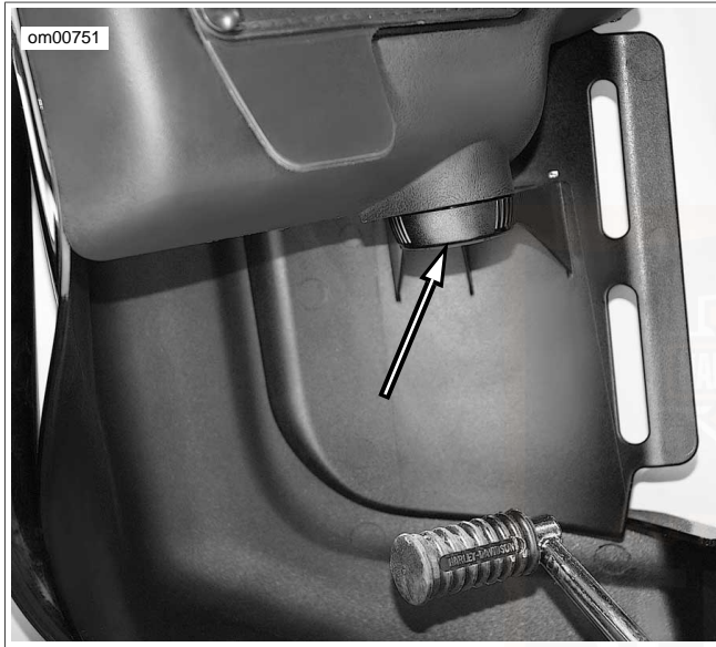
Figure 22. Fairing Lower Vent Control
