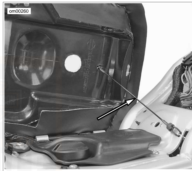
Figure 66. Seat Lanyard: VRSC Models
