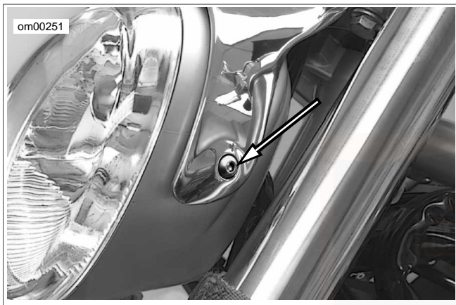
Figure 50. Headlamp Alignment Fastener: VRSC Models
