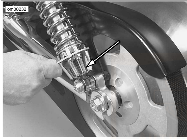
Figure 17. Adjusting Rear Shock: VRSC Models
