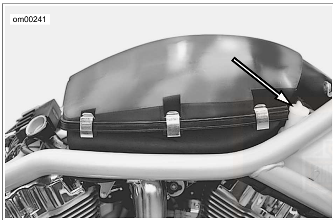
Figure 34. Expansion Tank Filler Cap
