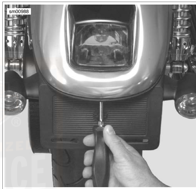
Figure 52. Releasing Tail Lamp Retaining Clip: VRSCAW/VRSCDX
