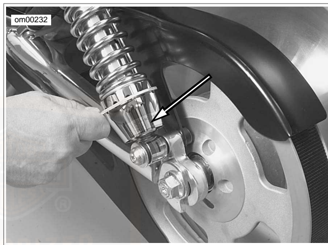
Figure 12. Rear Shock Absorber Adjustment: VRSCAW/VRSCDX Models
