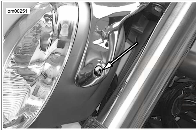
Figure 49. Headlamp Alignment Fastener: VRSCAW/VRSCF Models
